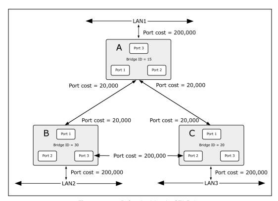
Figure 4-3-8-2: Before Applying the STA Rules
