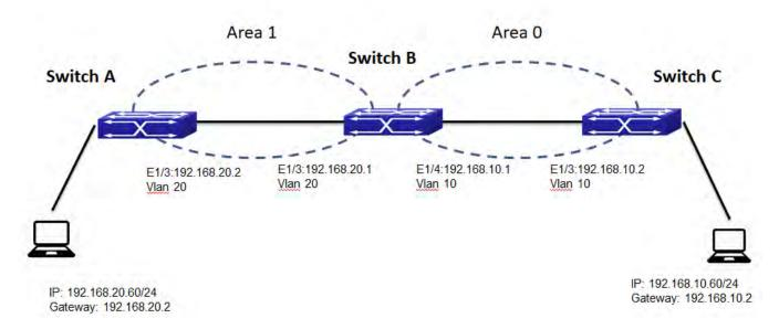
Figure 4-10-4-13 Network topology of OSPF autonomous system
