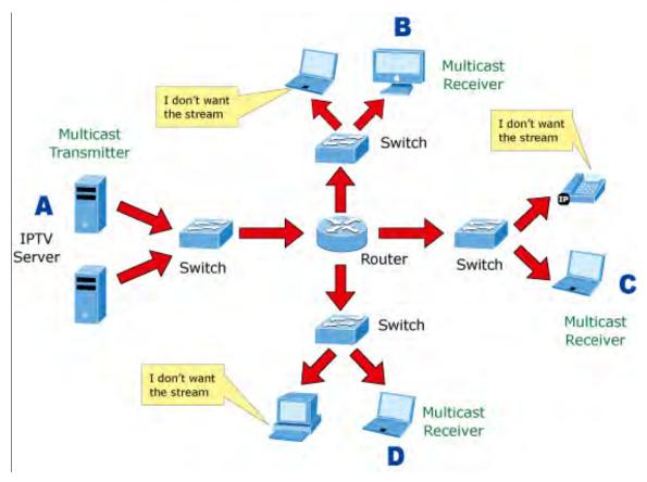
Figure 4-3-9-2: Multicast Flooding
