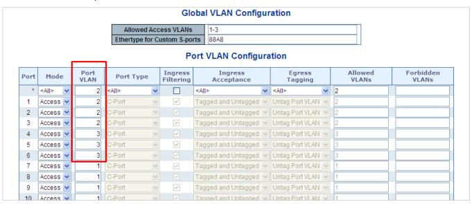
Figure 4-3-3-9: Change Port VLAN of Port 1~3 to be VLAN2 and Port VLAN of Port 4~6 to be VLAN3
