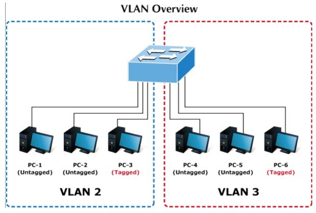
Figure 4-3-3-7: Two Separate VLANs Diagram
