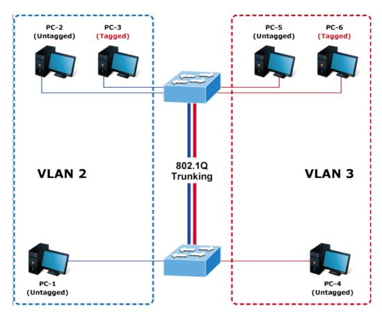
Figure 4-3-3-11: VLAN Trunking Diagram
