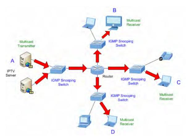
Figure 4-3-9-3: IGMP Snooping Multicast Stream Control
