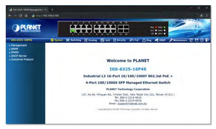
Figure 3-4: Web Main Screen of Industrial Managed Switch
